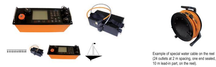
This set (completed with special water cables - not included in the set price) serves both for water level continuous measurement with GPS positioning and for borehole investigations (borehole-borehole, borehole-surface).
